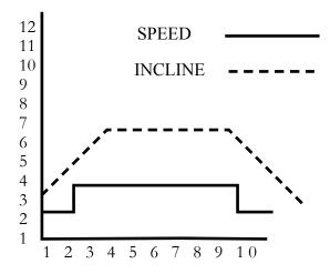
The **Warm Up Program** is designed to gradually increase the treadmill Speed and Elevation in the first segment (warm up) and gradually decrease the treadmill Speed and Elevation in the last segment (cool down). This is also known as a Plateau program.
